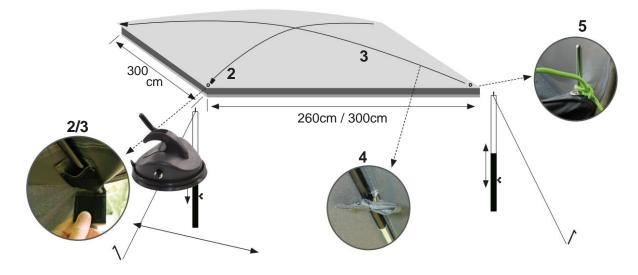
2/3: Insert fiberglass rods into the pocket on the vehicle and then on the opposite side. Insert the fi berglass bar into the pocket on the vehicle and then on the opposite side.
